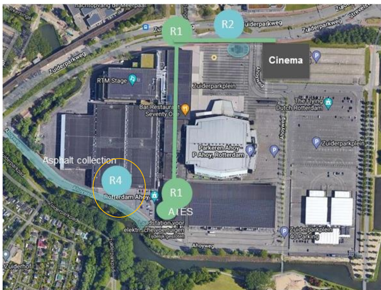
Figure 5: An overview of the Ahoy complex, RACC and cinema. All buildings connected by the main backbone (R1) and 2nd backbone to the cinema. R4 is situated next to the installation room of Ahoy (ATES)
